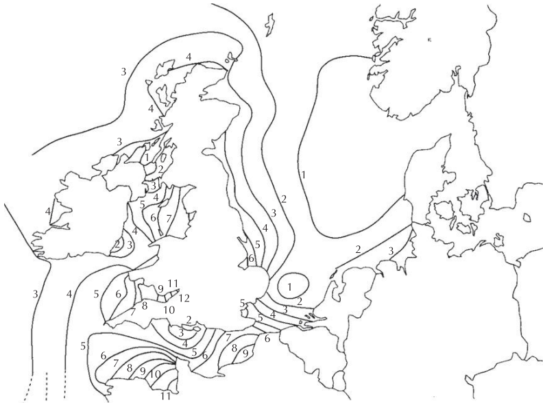
FIGURE 3.60 Tidal range H (difference between highest and lowest level in m) of the semi-diurnal lunar tides in the North Sea and adjacent straits. (Based on Kiilerich, 1965; Cavanagh et al. , 1993.)
