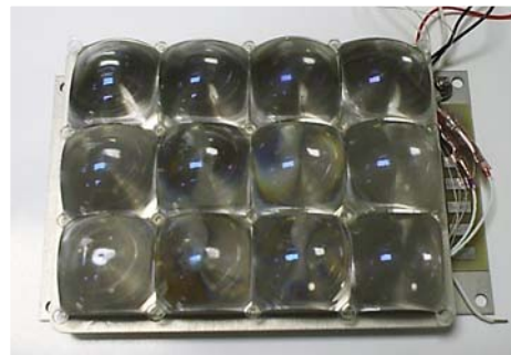
Figure 1.2: Photograph of PV Advanced Space Power (PASP+) module fabricated at Boeing using GaAs/GaSb stacked two-junction cells and flown in space by NASA in 1994 [22].
