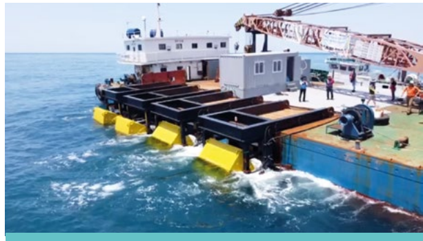
Actual sea demonstrations for rotor and hydraulic PTO system of (Courtesy: KRISO)
