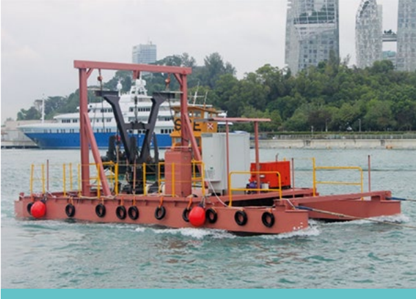
ERI@N developed Tidal turbine system
