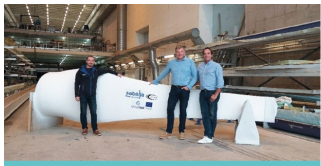
Optimized composite blade for Sabella's new generation of turbines
