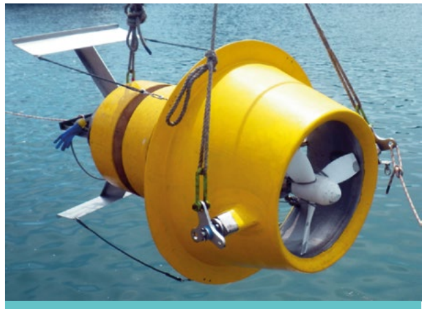
Nagasaki University tidal current power generator (Dimensions: L = 2m , B = D = 1.25m , turbine diameter = 0.64m )
