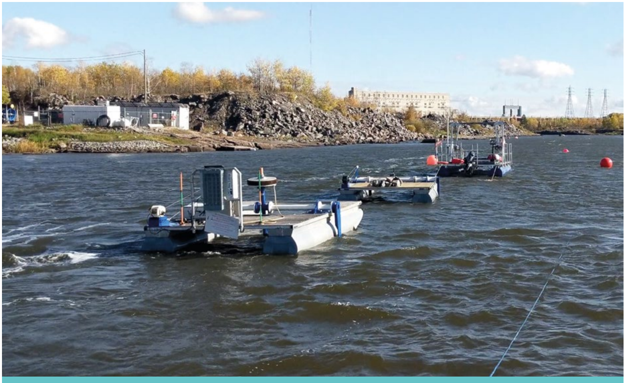
River hydrokinetic turbines testing being conducted at CHTTC
