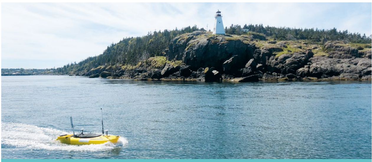
Jetyak in Petit Passage for an OERA funded project - a collaboration between Luna Sea Solutions, Dalhousie Ocean Acoustics Laboratory, and Memorial University to develop and validate software for detecting fish using Acoustic Doppler Current Profilers (ADCP)
