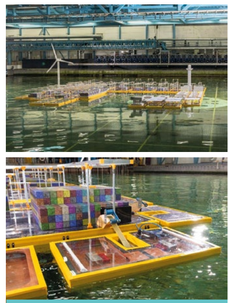
Tank testing of a modular floating island, WEC module with PTO. ©MARIN
