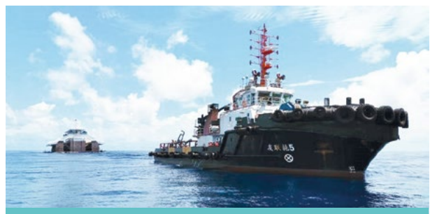
500 kW WEC "Zhoushan" towed by tugboats to the test sea area
