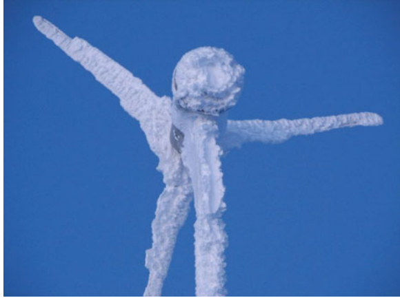
Fig. 4.9 Example of freezing on small size turbine. presented at HS seminar (Swedish Wind Energy Association), Stockholm, March 26, 2012, reproduced in the Presentation of Gran Ronsten (WindREN) with courtesy of Polar Field Services
