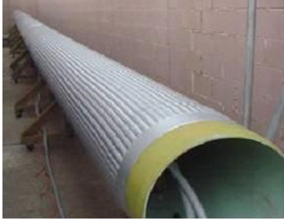
Fig. 5.40 Pneumatic de-icing system, picture of the experimental rig [25]
