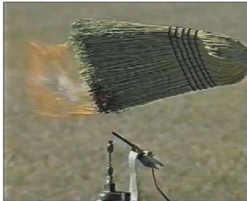
Figure 1-8 Invisible Hydrogen Flame Igniting Broom
