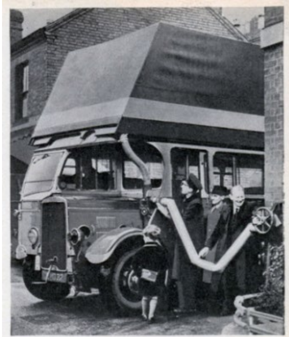
Gas Bag on Roof Holds Bus Fuel
