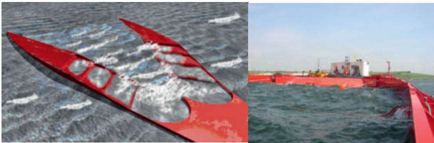
Figure 4: Overtopping wave power technologies: WaveCat (left) and Wave Dragon (right).
