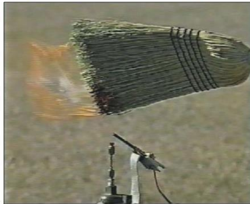
Figure 1-8 Invisible Hydrogen Flame Igniting Broom.
