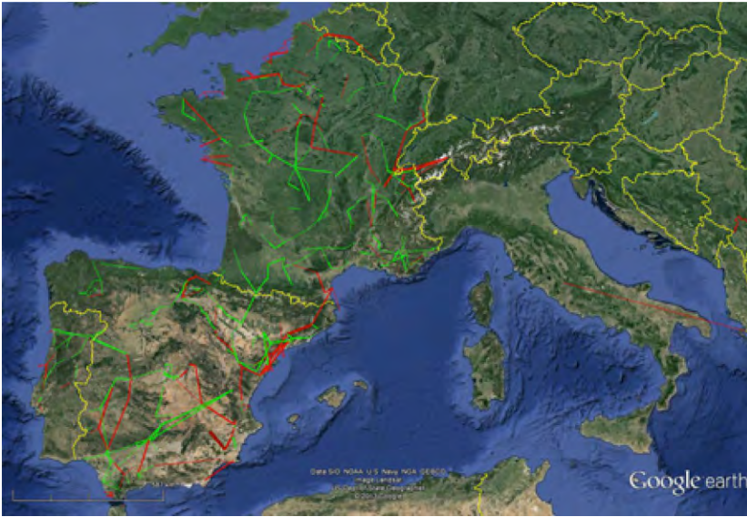
FIG. 7.2 Optimal network, with 220kV lines represented in green (light grey) and 400kV or HVDC represented in red (dark grey).
