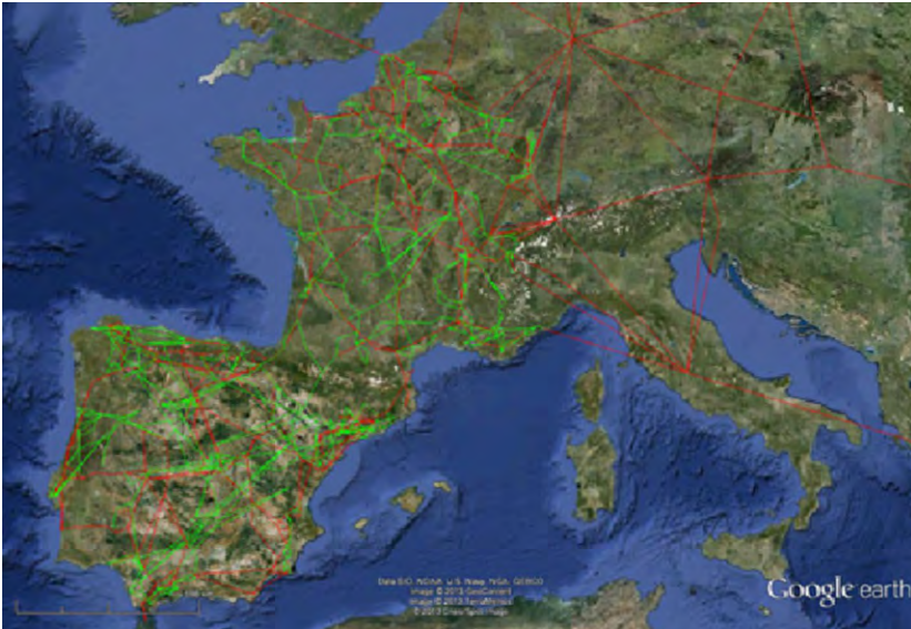
FIG. 7.1 Initial network. Green (light grey) is used for 220kV (only for Spain, France, and Portugal) and red (dark grey) for 400kV lines and HVDC.
