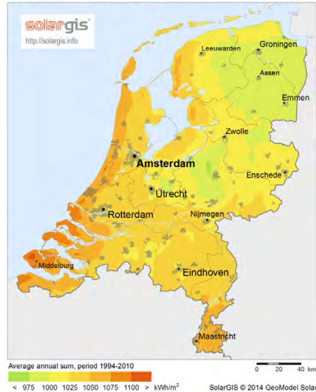
Figure 18.3: The average global horizontal insolation of the Netherlands given in kWh/year and PSH/day [101].
