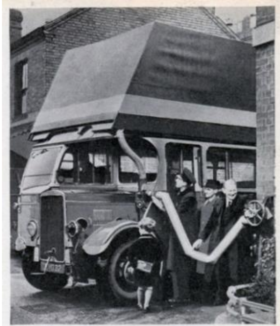
Gas Bag on Roof Holds Bus Fuel
