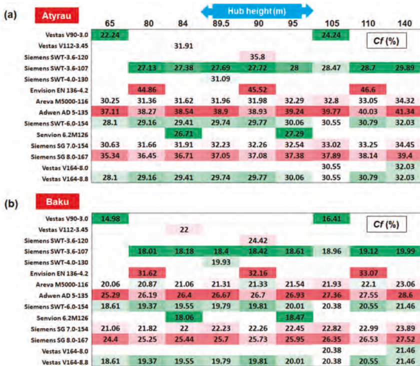
Figure 10. The capacity factor (%) reported for the full time distribution, considering the sites: (a) Atyrau; (b) Baku. The points are located at a distance of 5 km from the shoreline.
