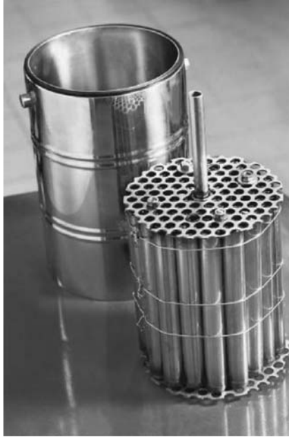
Figure 9.40 Heat recovery system for exhaust gases from a diesel engine. The heat exchanger and its casing work as a latent TES (Kauranen et al. , 2010)
