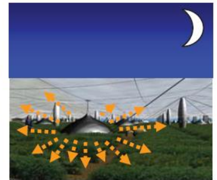
Night water bags release sun heat
