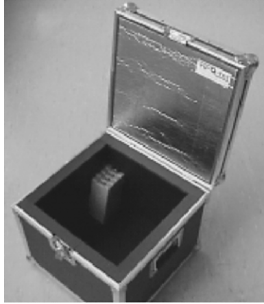
Figure 124. Transport box from Va-Q-tec. Due to the vacuum super insulation a cooling power of less than 10 W by a PCM is sufficient to sustain -20\text{ }^{\circ}\text{C} for 4 days in the box in a +30\text{ }^{\circ}\text{C} environment (picture: Va-Q-tec GmbH)
