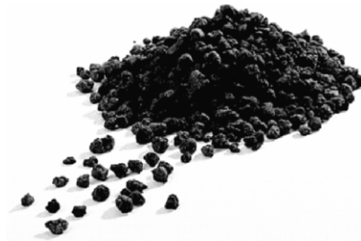
Figure 123. PCM-graphite compound produced from mixing PCM with expanded graphite
