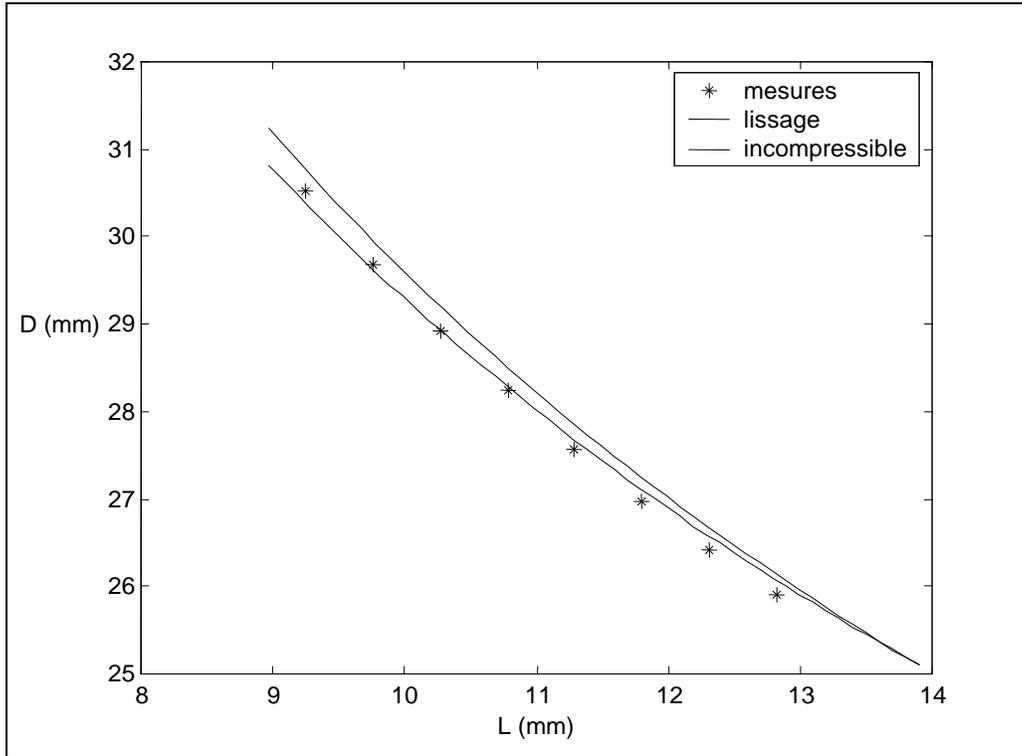
Coefficient de Poisson (lissage) = 0.46895,  $R^2 = 0.86859$
